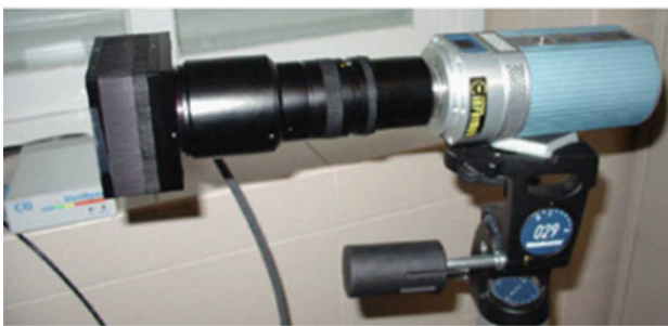
Hyperspectral Imaging, Fig. 3 (Left) CCD monochrome camera coupled with an LCTF placed in front of the lens of the camera; (right) spectral sensitivities of the channels selected in the LCTF [9]
