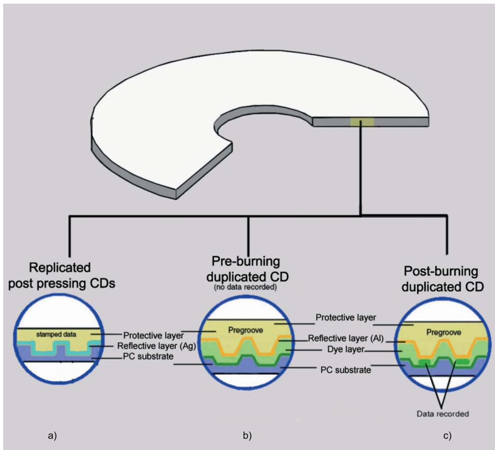
Fig. 4. A schematic cross section of (a) a replicated CD, (b) blank recordable CD-R, and (c) a burned CD-R.
