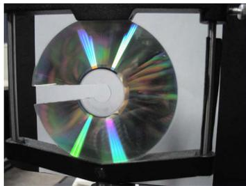
Fig. 2. Photograph of a CD used in the experiment. The missing segment was used in the scanning electron microscope study.
