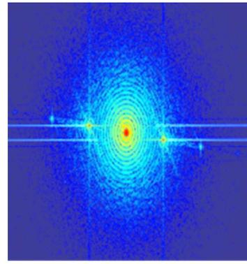
Fig. 6. Simulation of Fraunhofer diffraction using the reflectance of a burned CD-R surface and Eq. (3). In this simulation we assumed the use of a 633 nm He-Ne laser.
