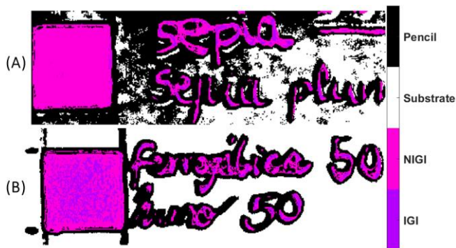
Figure 3. Classification maps of two minicubes: (A) sepia ink, and (B) mixture of iron gall ink and lamp black 50:50, both applied on cotton-linen paper.
