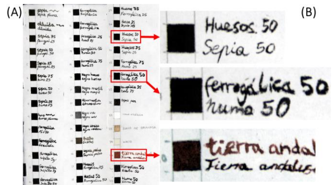
Figure 1. False RGB images ([605, 535, 430] nm) of laboratory samples in cotton paper. (A) Full pages; (B) Extracted minicubes.
