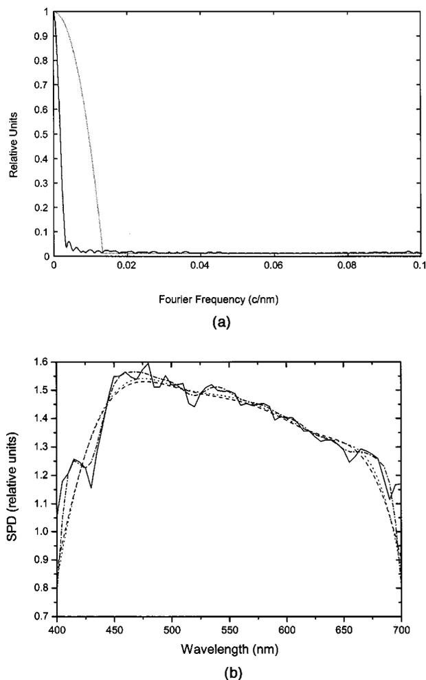
Fig. 3. (a) FFT of daylight SPD and parabolic filter of 0.02 c/nm: solid curve, SPD; dotted curve, parabolic filter. (b) Daylight SPD and three filtered signals obtained with a parabolic filter with three different cutoff frequencies: solid curve, original; dotted-dashed curve,  $f = 0.04$  c/nm; dotted curve,  $f = 0.016$  c/nm; dashed curve,  $f = 0.013$  c/nm.
