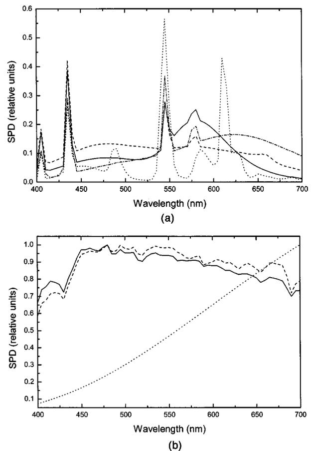
Fig. 2. (a) SPDs of the fluorescent illuminants used: solid curve, F2; dashed curve, F7; dotted curve, F11; dotted-dashed curve, commercial fluorescent. (b) Two examples of daylight SPD and CIE illuminant A: solid curve, daylight 1; dashed curve, daylight 2; dotted curve, A.
