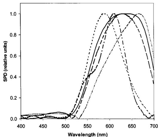
Fig. 6. Normalized SMSF-filtered signals for object v142 (see Ref. 23) and five different illuminants: solid curve, daylight; long dashed, commercial fluorescent; short dashed, F1; heavy dotted-dashed, F10; light dotted-dashed, A.
