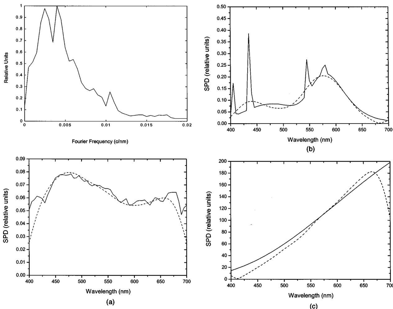
Fig. 5. Original (solid curve) and filtered (dashed curve) signals obtained with the SMSF filter: (a) daylight; upper panel, normalized SMSF filter (see Ref. 10); (b) F2 fluorescent; (c) illuminant A.
