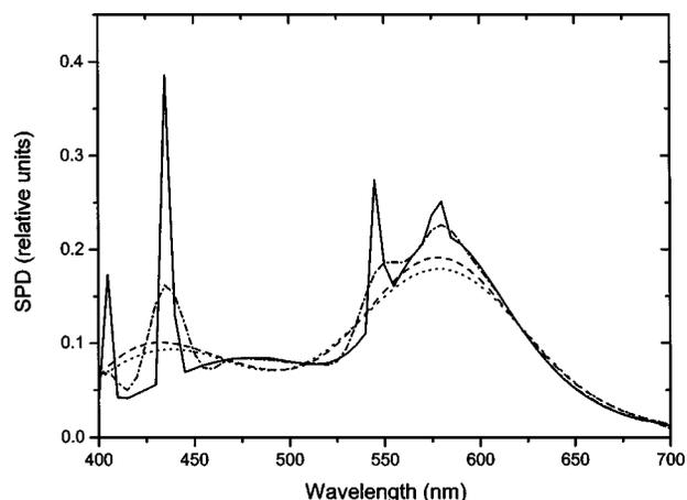
Fig. 4. SPD of the illuminant F2 and three filtered signals obtained with a parabolic filter with three different cutoff frequencies: solid curve, original; dotted-dashed curve,  $f = 0.04$  c/nm; dashed curve,  $f = 0.016$  c/nm; dotted curve,  $f = 0.013$  c/nm.
