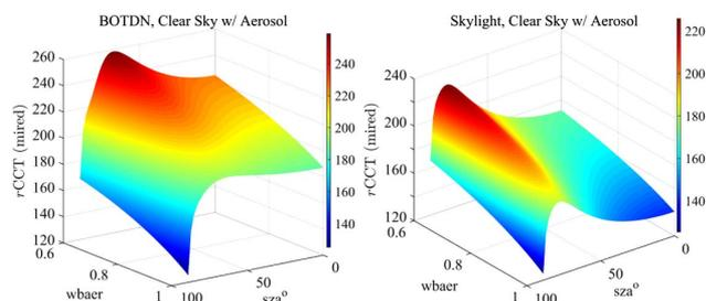
**Fig. 8.**  $r\text{CCT}$  of BOTDN and skylight in a clear sky with aerosol particles, simulated as a function of solar zenith angle,  $\text{sza}$ , and single scattering albedo,  $\text{wbaer}$ .
