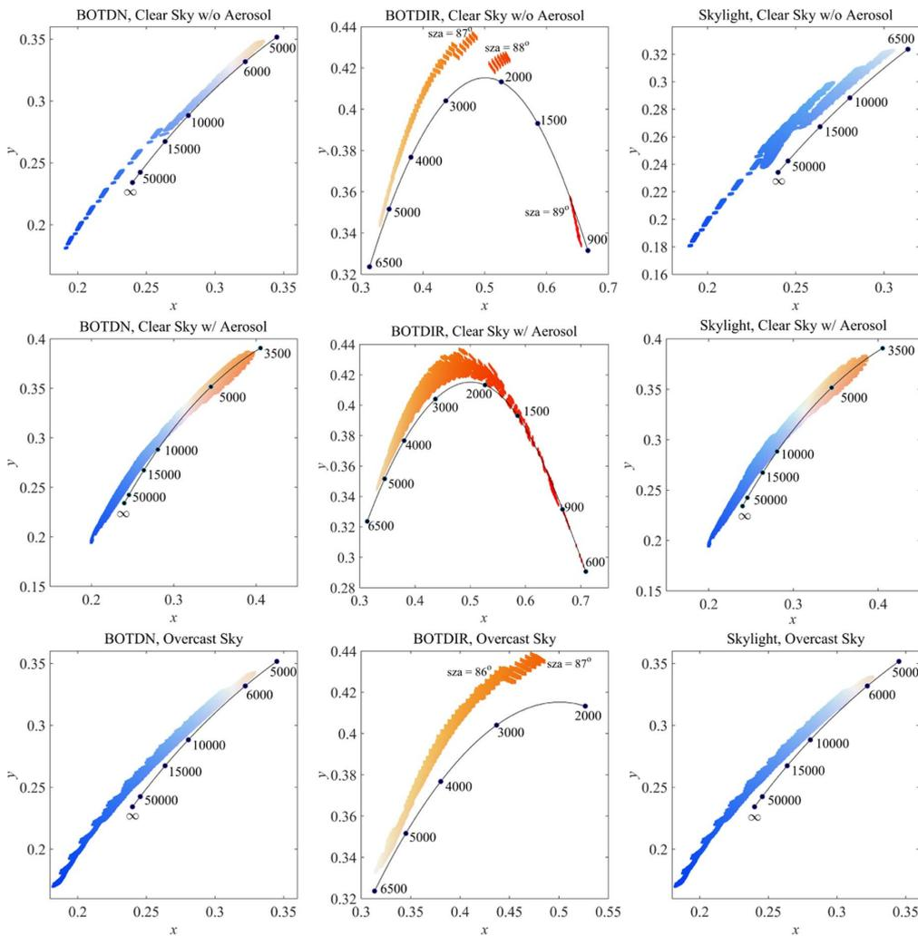
**Fig. 5.** CIE 1931 chromaticity diagram of daylight (BOTDN), direct sunlight (BOTDIR), and skylight irradiance functions simulated under the atmospheric conditions of clear sky without aerosol particles, clear sky with aerosol particles, and overcast sky.
