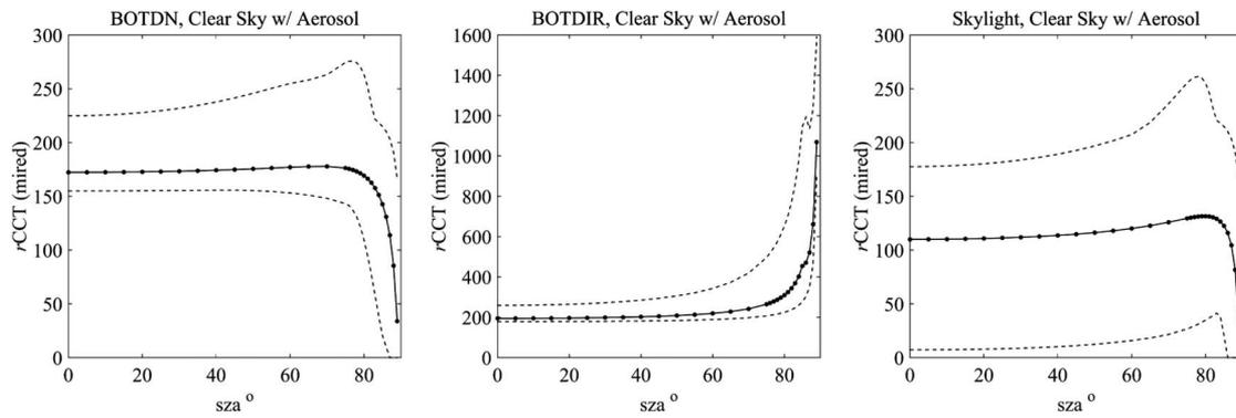
**Fig. 3.** Average  $rCCT$  (mired) of daylight (BOTDN), direct sunlight (BOTDIR), and skylight irradiance functions simulated under the atmospheric conditions of clear sky with aerosol particles as a function of solar zenith angle ( $sza^\circ$ ). In this figure, the dashed lines show the observed minimum and maximum limits of the  $rCCT$  values.
