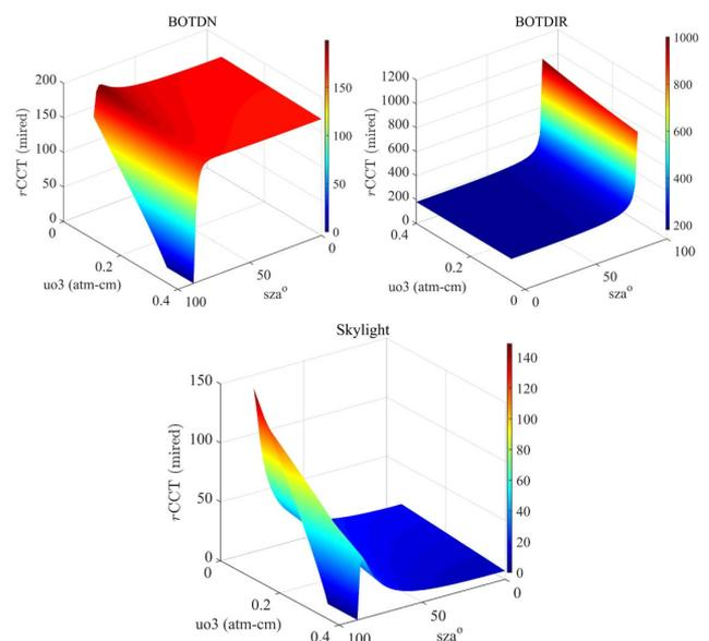
**Fig. 7.**  $rCCT$  of BOTDN, BOTDIR, and skylight in a clear sky without aerosol particles, simulated as a function of solar zenith angle,  $sza$ , and ozone concentration,  $uo_3$ .
