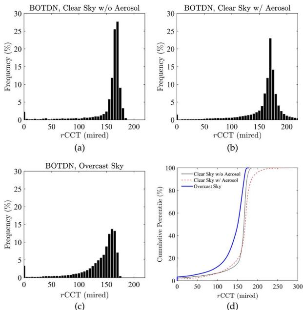
**Fig. 4.** Histogram of  $rCCT$  for daylight (BOTDN) under the atmospheric conditions of (a) clear sky without aerosol particles, (b) clear sky with aerosol particles, and (c) overcast sky. The bin size is 5 mired wide in each histogram. (d) The plots of cumulative percentile of the  $rCCT$  under the three atmospheric conditions.
