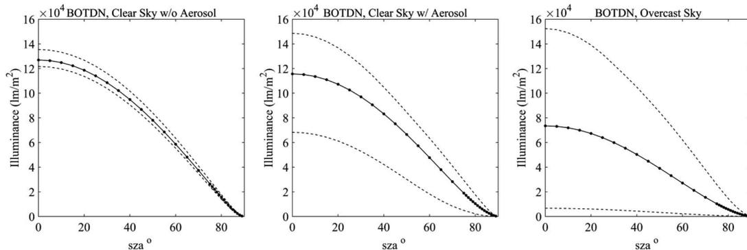
**Fig. 2.** Average illuminance values of hemispheric daylight (BOTDN) simulated under the atmospheric conditions of clear sky without aerosol particles, clear sky with aerosol particles, and overcast sky are presented as a function of solar zenith angle ( $\text{sza}^\circ$ ). In this figure, the dashed lines show the observed minimum and maximum limits of the illuminance values.
