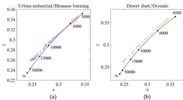
**Fig. 9.** CIE 1931 chromaticity diagram of hemispheric daylight simulated by parameters introduced in Table 4. (a) Chromaticities in the atmosphere with urban–industrial/biomass burning aerosols are mainly located above the Planckian locus at CCT > ~10,000 K, with a slight shift toward the purple side at lower CCTs. (b) Chromaticities of simulated daylight in the oceanic atmosphere with desert dust and higher amounts of water vapor are all located above the Planckian locus.
