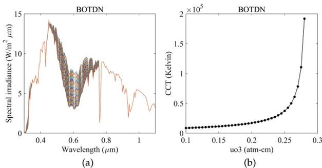
**Fig. 6.** (a) Simulated daylight spectral irradiance (BOTDN) of a typical overcast sky during twilight with different amounts of ozone concentration. (b) The CCT of the simulated spectra as a function of ozone concentration,  $uo_3$ , within the range of 0.1–0.28 atm-cm.
