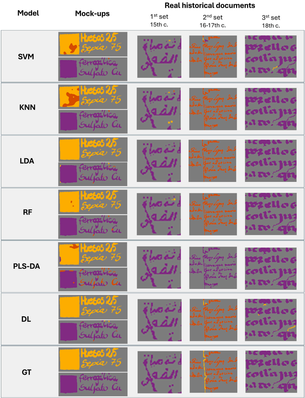
Fig. E.10. Classification maps obtained using all the models studied (SVM, KNN, LDA, RF, PLS-DA, and DL) after cleaning post-processing. The Ground Truth (GT) images are shown in the last row. Purple: metallo-gallate ink (MGP); yellow: carbon-containing ink (CC); orange: non-carbon-containing ink (NCC).
