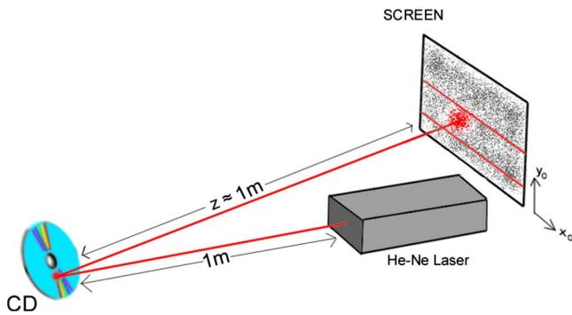
Fig. 1. The Fraunhofer diffraction experiment used to distinguish between replicated and duplicated compact discs. Although it is not shown clearly in the diagram, the angle of incidence is roughly normal and the screen is parallel to the surface of the disc. In this arrangement only the zero-order diffracted image is visible in the photographs (see Fig. 3). If the screen were moved closer to the CD, higher orders would become visible.
