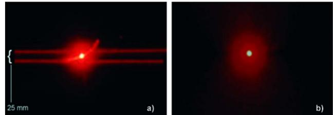
Fig. 3. Diffracted laser light patterns for (a) a burned CD and (b) a pressed CD. The diffraction patterns were photographed by a digital camera. In both cases the tracks are vertical and only the zero-order diffracted image is visible in the photograph.
