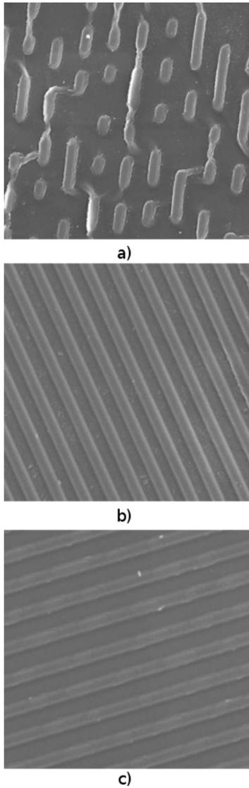
Fig. 5. Scanning electron microscope images of the surfaces of (a) a pressed CD, (b) a blank CD-R, and (c) a burned CD-R. The bar in the bottom left-hand corner of each image corresponds to  $1\ \mu\text{m}$  in the CD's surface.
