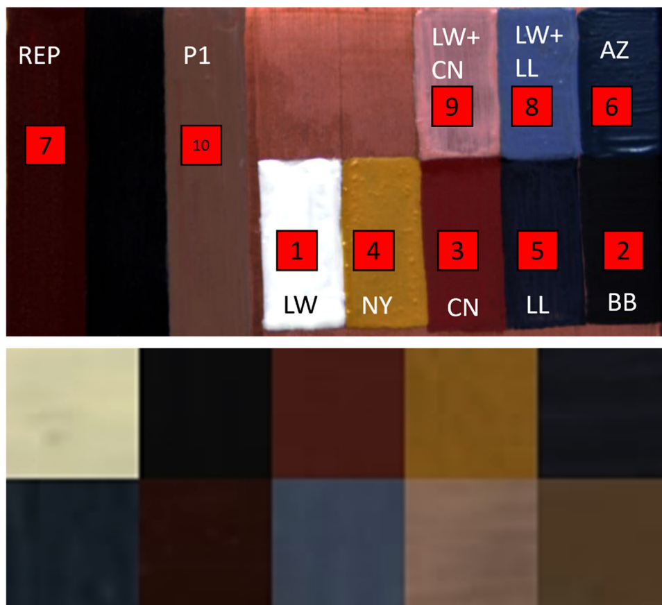
Fig. 1. (Top) Reference copper plate. Reference checker areas extracted are highlighted with red squares. (Bottom) Reference checkerboard image containing areas 1–10 (for interpretation of the references to color in this figure legend, the reader is referred to the web version of this article).
