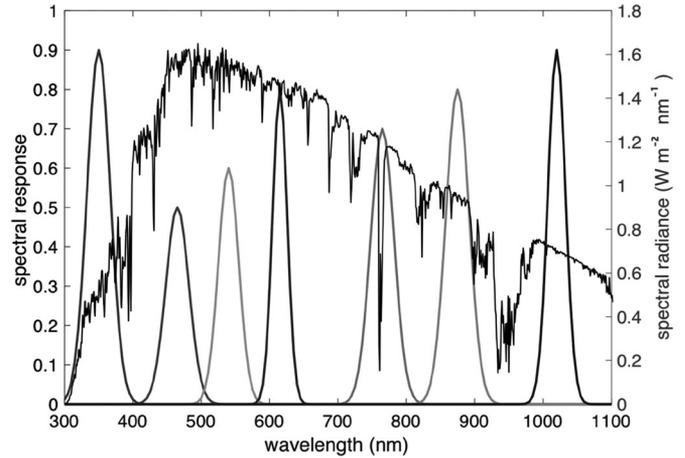
Fig. 4. Spectral responses of an optimum set of seven sensors (left axis) superimposed to the ASTM global tilt reference spectrum (right axis).
