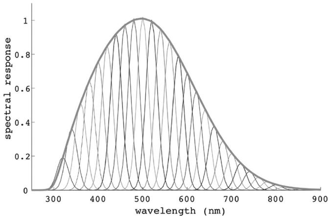
Fig. 2. Example of how a system of 28 sensors, whose spectral responses have an FWHM of 30 nm and whose peak central wavelengths are separated 40 nm, can be used to emulate the response of an a-Si PV cell.
