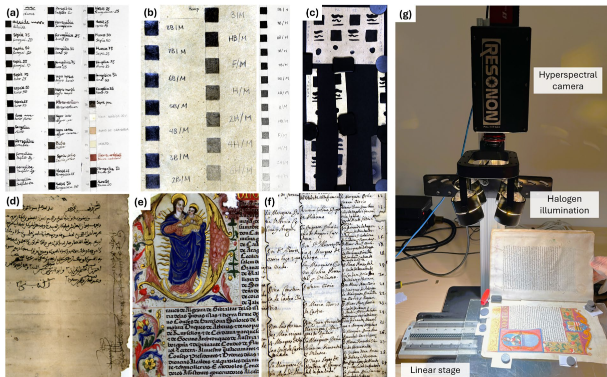
Fig. 2 Examples of samples from different subsets: (a) mock-ups of historical inks on cotton paper, (b) pencil mock-ups, (c) mock-ups of artificially aged metallo-gallate inks, (d) manuscript of the Provincial Historical Archive of Granada, (e) illuminated manuscript from the Archive of the Royal Chancellery of Granada, (f) family tree from the Archive of the Royal Chancellery of Granada; and (g) hyperspectral capture using the Pika IR+ camera.
