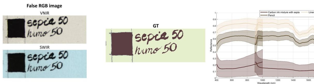
Fig. 10 False-color RGB images (left) created using bands [645, 565, 440] nm (top) and [1700, 1300, 1100] nm (bottom), Ground Truth (GT) image (center), and the mean spectral reflectances with standard deviation for the labels present in the GT, extracted from the minicubes '00007-VNIR-mock-up.h5' and '00007-SWIR-mock-up.h5' (right).
